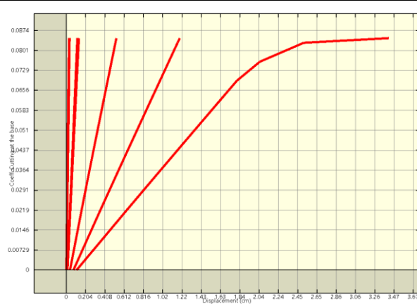
Pushoveranalysis"Pushover-X Acc": capacitycurve.
